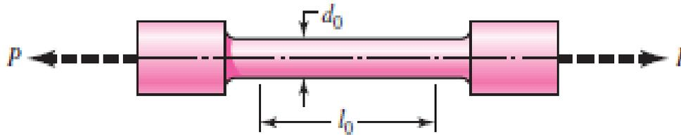
**Fig 2.1 Typical tension-test specimen.**
