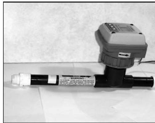
Turbine used for measurement of volume flow rate of water flowing in a pipe
