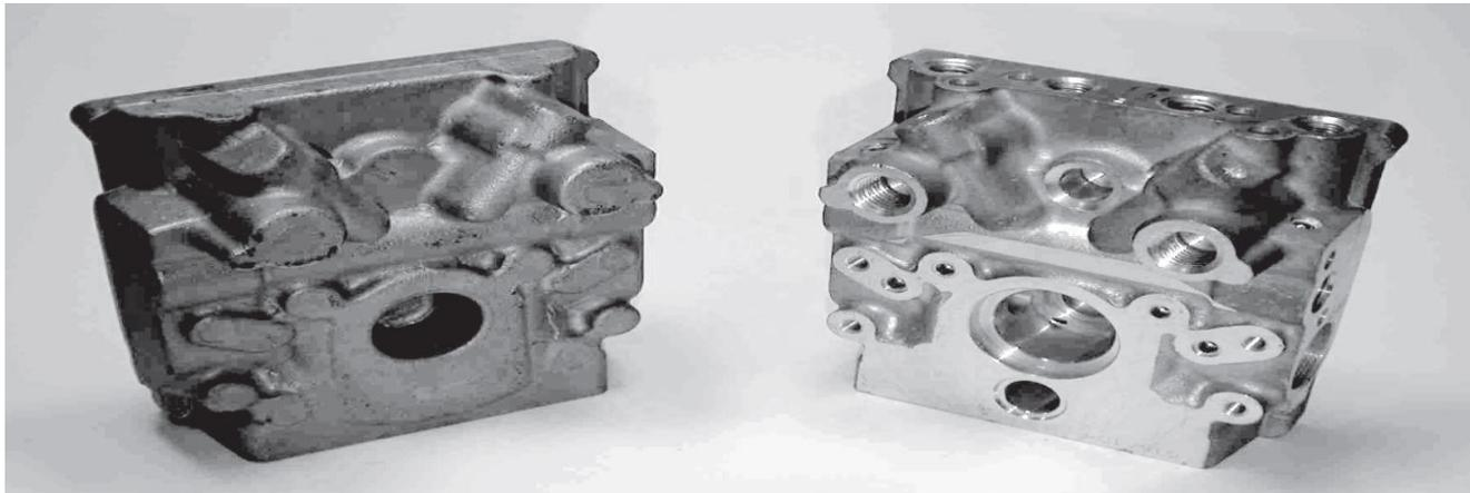
FIGURE 4: This body for a hydraulic valve assembly was first cast from aluminum (left) and then machined in order to produce holes, flatten surfaces, and cut threads (right).
