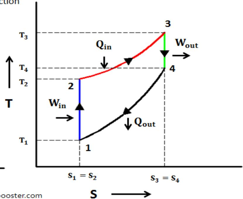
**P-V and T-S Diagram of Diesel Cycle**
