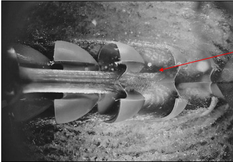
The buckets are shaped carefully to take advantage of the high momentum water jet, and are designed to turn around the water nearly  $180^\circ$  for maximum transfer of momentum from the water jet to the rotating turbine wheel.
